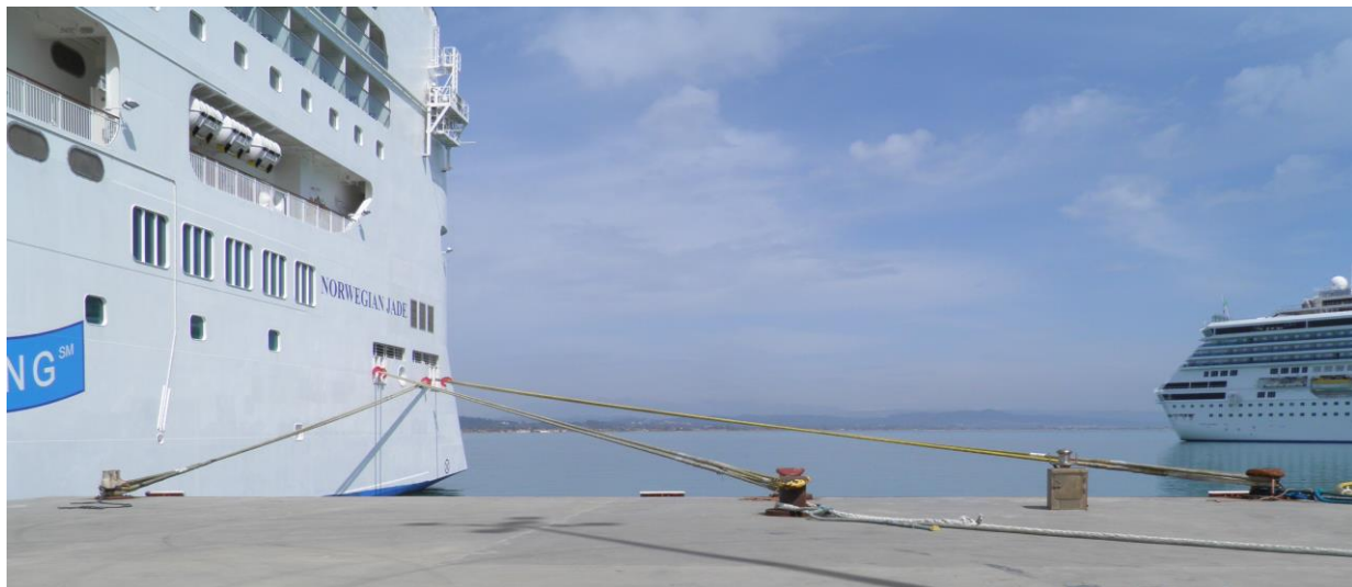
Figure 24. Port stern quarter mooring configuration.
